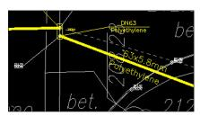
The generation of drawings of external gas system as regards pipeline routes, shut-off fittings, locations and dimensions of free-standing and wall-mounted gas
